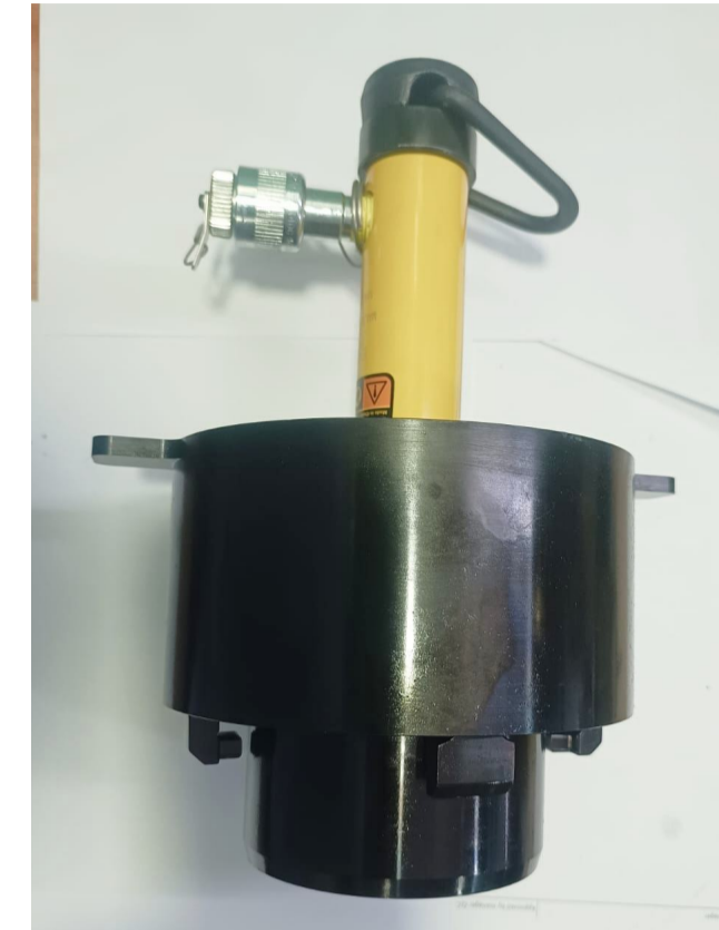
FIXTURE REMOVE-NO 04 SEAL RUNNER
